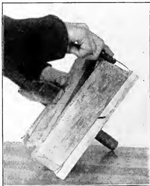
Fig. 202—Rails and Shelf Clamped Together
